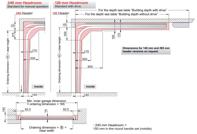
Please observe the following measurement details to guarantee exact assembly and precise and reliable operation of the CarTeck sectional door.
